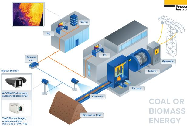
The ThermoView software allows for quick setup of Areas of Interest (AOIs) for conditions to only trigger alarms when temperatures are outside of set parameters and additional functionality allows for narrowing the alarm window. For example you could set AOIs to alarm only when >30% of an area exceeds a potential hot spot temperature threshold. An on-screen dimensional reference tool also allows for material level estimation.
